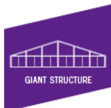
Generally defined as large span aluminium frame or tensioned pole tents that are in excess of 25m wide. These can be 30/40/50m span frame tents usually needing the aid of telescopic plant or cranes to erect and dismantle. Giant pole tents can usually be erected manually, thus differentiating them from Big Tops that require plant.
